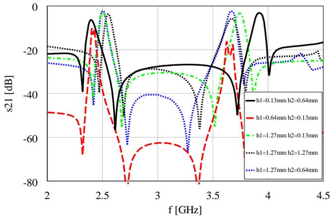
Fig. 7. Influence of the substrate thicknesses to the dual-band dual-mode filter characteristic.
