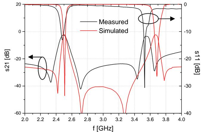
Fig. 9. Measured and simulated responses of the proposed filter
