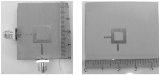
Figure 8. Photograph of the fabricated dual-band dual-mode filter.
