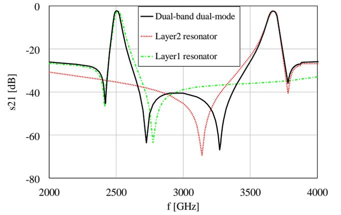
Fig. 3. Simulation results for two dual-mode resonators and the proposed dual-band dual-mode filter.
