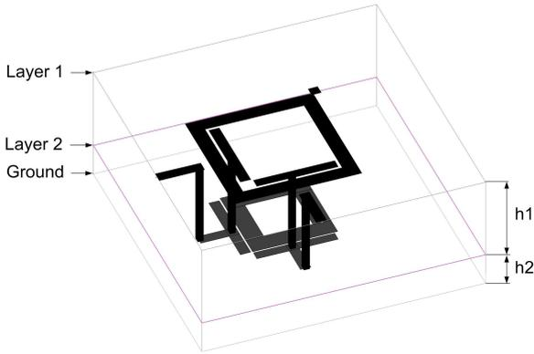
Fig. 2. 3-D view of the proposed dual-band dual-mode filter (for clarity, ground is not shown in separate color).
