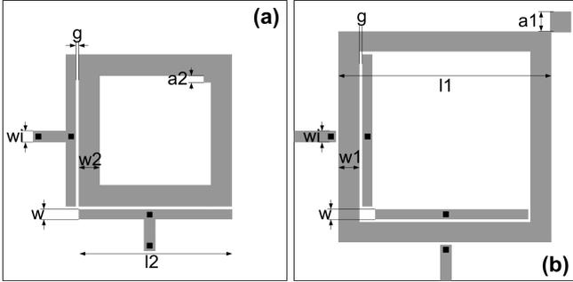
Fig. 1. Layout of the filter: (a) middle conductive layer (layer2), (b) top conductive layer (layer1)
