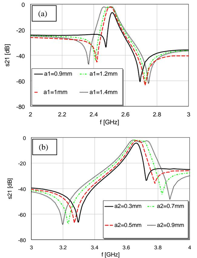
Fig. 4. Influence of the perturbations size to dual-band dual-mode characteristic: (a) influence of  $a_1$  for  $a_2$  fixed, (b) influence of  $a_2$  for  $a_1$  fixed
