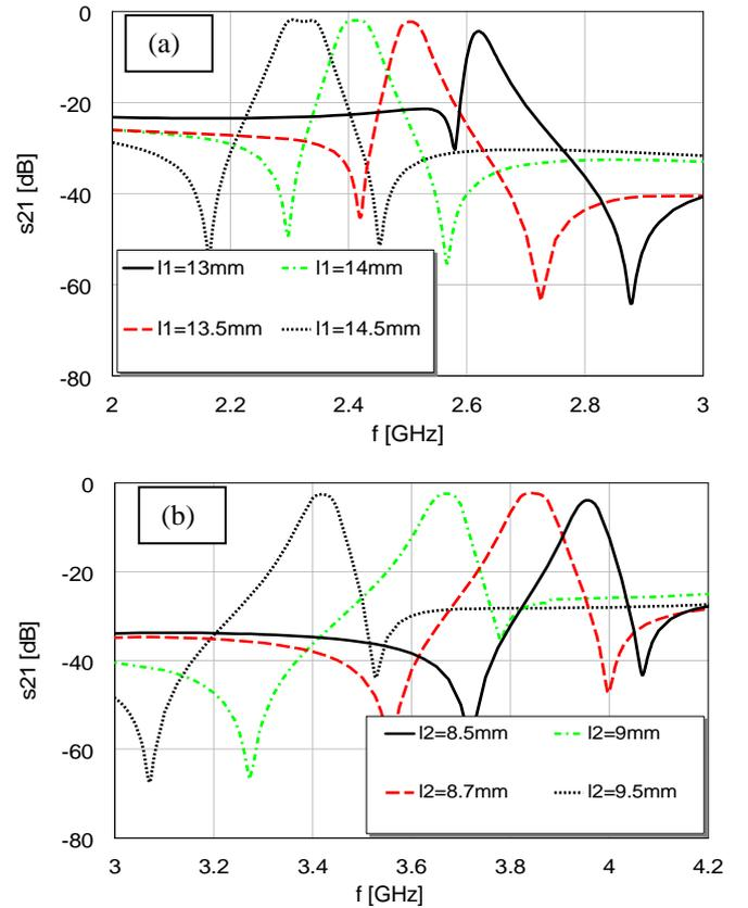
Fig. 6. Influence of the loop size to filter characteristic: (a) influence of  $l_1$  for  $l_2$  fixed, (b) influence of  $l_2$  for  $l_1$  fixed
