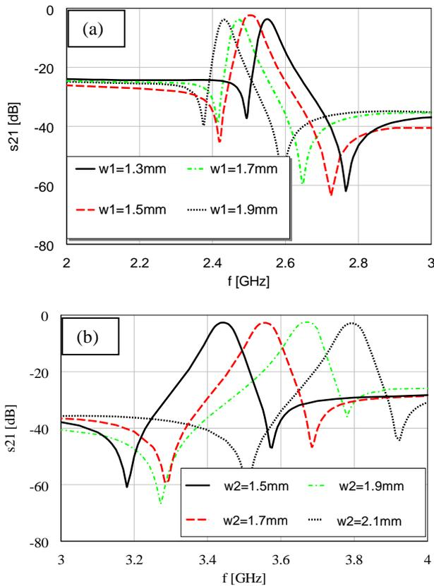
Fig. 5. Influence of the loop line width to dual-mode dual-band filter characteristic: (a) influence of  $w_1$  for  $w_2$  fixed, (b) influence of  $w_2$  for  $w_1$  fixed
